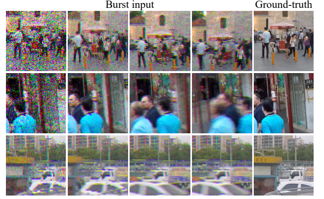
Figure 4. Visualization of DEB. The left four columns display a subset of 14 input bursts, while the rightmost column is the ground-truth image. From the left to the right in burst, the exposure time increases.
